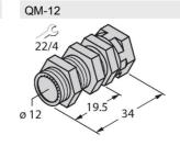
Quick-mount bracket with dead-stop; material: Chrome-plated brass. Male thread M16 × 1. Note: The switching distance of the proximity switches may change when using quick-mount brackets.
