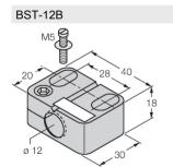
6947212 Mounting clamp for threaded barrel sensors, with dead-stop; material: PA6
