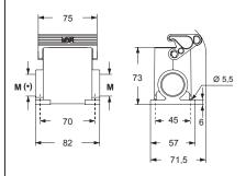
(•) The surface mounting, high construction housings are supplied with an open threaded entry (•) and diametrically opposite a closed threaded entry which can be opened by the user if required (with suitable tool).
