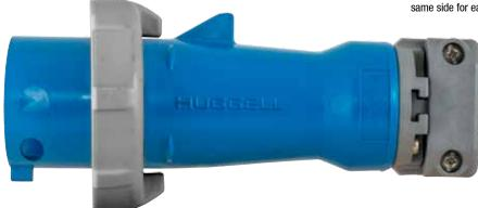
Male locking rings include torque tabs to help facilitate proper engagement of the gasket for maximum environmental protection UV-stabilized, impact and chemical-resistant PBT housing
