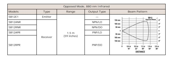
Standard 2 m (6.5 ft) cable models are listed. QD Models: For 3-Pin 150 mm (6 inch) pigtail with threaded Pico-style M8 connector, add suffix "Q3" to the model number (e.g. SB12E1Q3).
