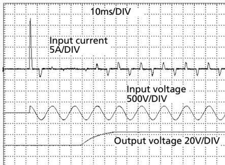
Fig. 5-2 Input inrush current, zoom into first peak
