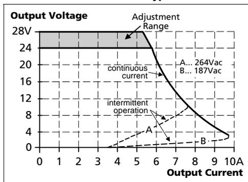
Fig. 6-2 **Intermittent operation at shorted output, typ.**
