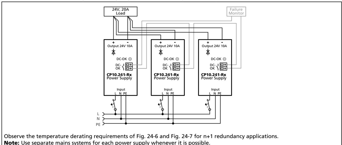
Observe the temperature derating requirements of Fig. 24-6 and Fig. 24-7 for n+1 redundancy applications.
