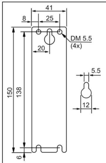
Fig. 23-6 **Wall/panel mounting, side view**
