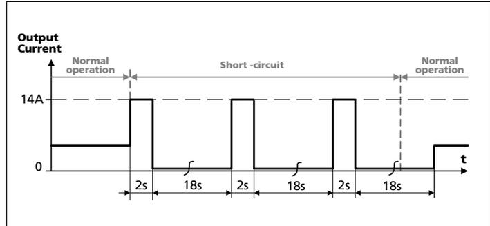
Fig. 6-3 Dynamic overcurrent capability, typ.
