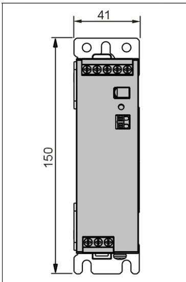
Fig. 23-5 **Hole pattern for wall mounting**
