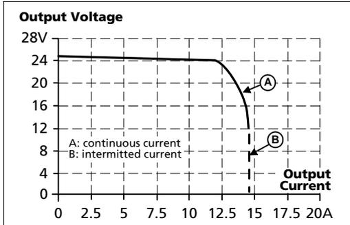
Fig. 6-2 Short-circuit on output, Hiccup<sup>PLUS</sup> mode, typ.
