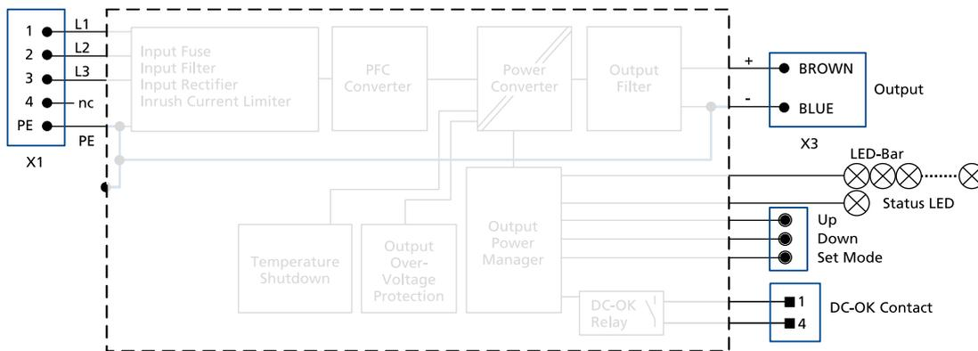
Fig. 12-2: Functional Diagram FPT500.241-006-104
