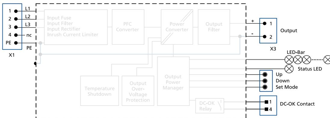
Fig. 12-3: Functional Diagram FPT500.241-010-108
