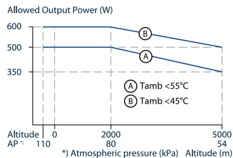
Fig. 16-2: Output power vs. ambient temp.
