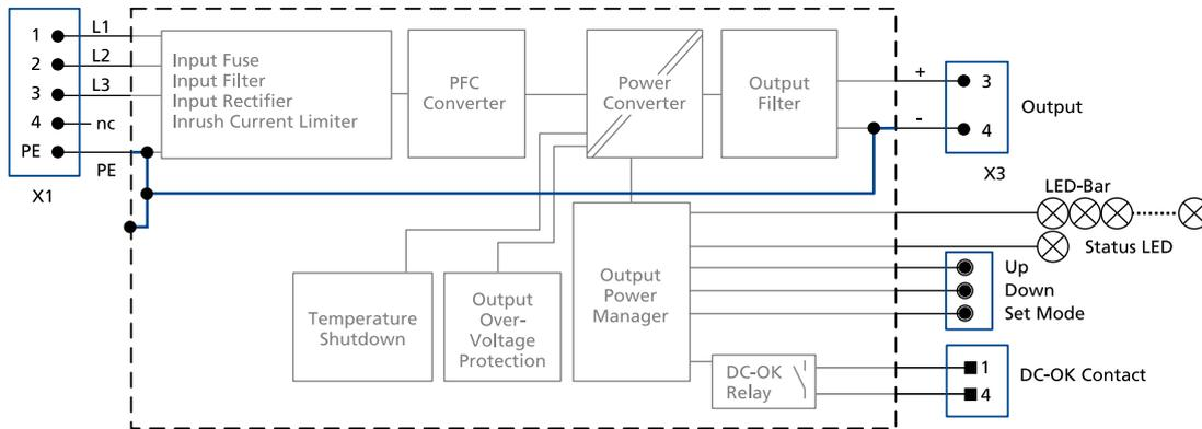
Fig. 12-1: Functional Diagram FPT500.241-002-101
