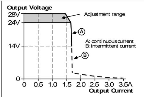
Fig. 6-2 Intermittent current at short circuit, typ.
