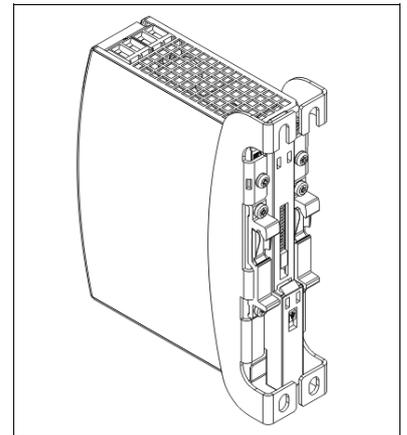
Fig. 22-4 Wall/panel mounting, front view
