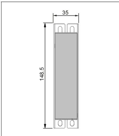
Fig. 22-5 Hole pattern for wall mounting
