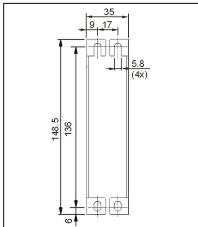
Fig. 22-6 Wall/panel mounting, side view
