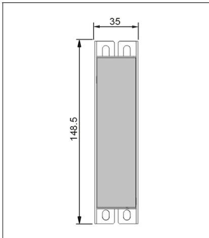
Fig. 22-5 **Hole pattern for wall mounting**
