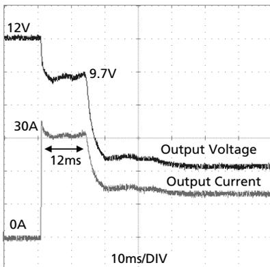
Please note: The DC-OK relay triggers when the voltage dips more than 10% for longer than 1ms.
