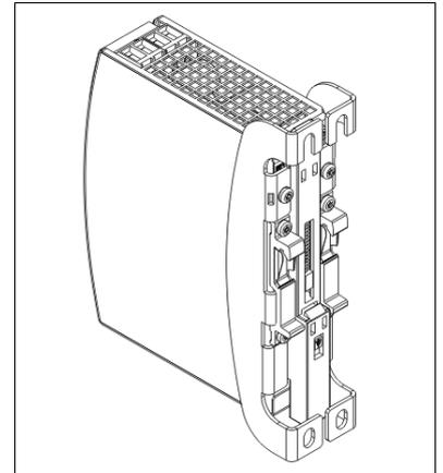
Fig. 22-4 **Wall/panel mounting, front view**
