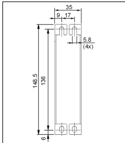
Fig. 22-6 **Wall/panel mounting, side view**
