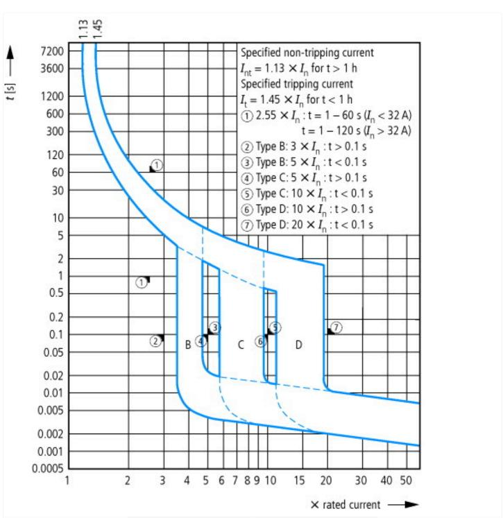
Tripping characteristic at 30 °C: S according to IEC/EN 60947
