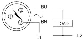
**WARNING: NO SHORT-CIRCUIT PROTECTION. ALWAYS WIRE A LOAD IN SERIES WITH THE SENSOR.**
