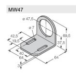
69452 Mounting bracket; material: Steel plate, galvanized
