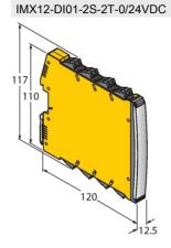
7580020 Isolating switching amplifier, 2-channel; SIL2 acc. to IEC 61508; Ex-proof version; 2 transistor outputs; input Namur signal; ON/OFF switchable monitoring of wire-break and short-circuit; toggle between NO/ NC mode; signal doubling; removable screw terminals; 12.5 mm wide; 24 VDC power supply
