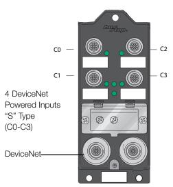
This busstop <sup>®</sup> station has four input connectors. Each connector provides one input. The LED at each input point turns green when the input is on. Inputs are protected against short-circuit as a group. If any input is shorted, the entire group of inputs are disconnected from bus power.
