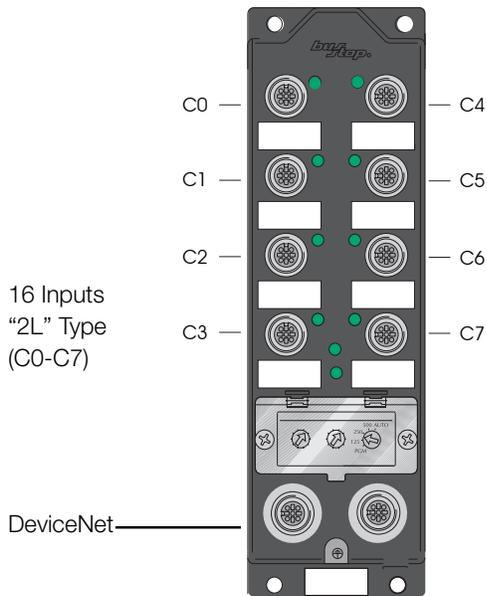
This busstop® station takes in up to sixteen discrete three-wire inputs or eight discrete four-wire input points per node. There are two inputs per connector—one on pin four and one on pin two. Each input automatically detects a sourcing (PNP) or sinking (NPN) open-collector signal. Any combination of NPN and PNP devices may be used.
