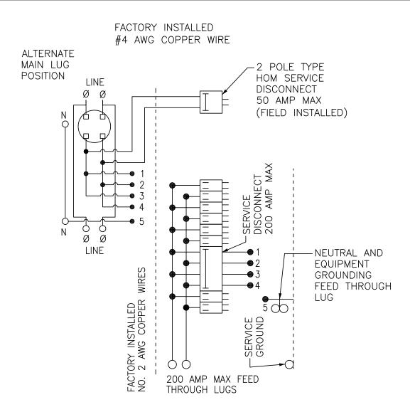
TWO SINGLE POLE, ONE PLUG-ON SPACE TYPE HOMT OR ONE SINGLE POLE, ONE PLUG-ON SPACE TYPE HOM. TWO POLE TYPE HOM, HOMA OR HOMT MAY PLUG-ON TWO ADJACENT SPACES. A 100 AMP MAX. CIRCUIT BREAKER MAY BE INSTALLED IN THE LOWEST POSITION IN THE BRANCH PANEL. ALL OTHER POSITIONS ARE LIMITED TO 70 AMP MAX. CIRCUIT BREAKERS.
