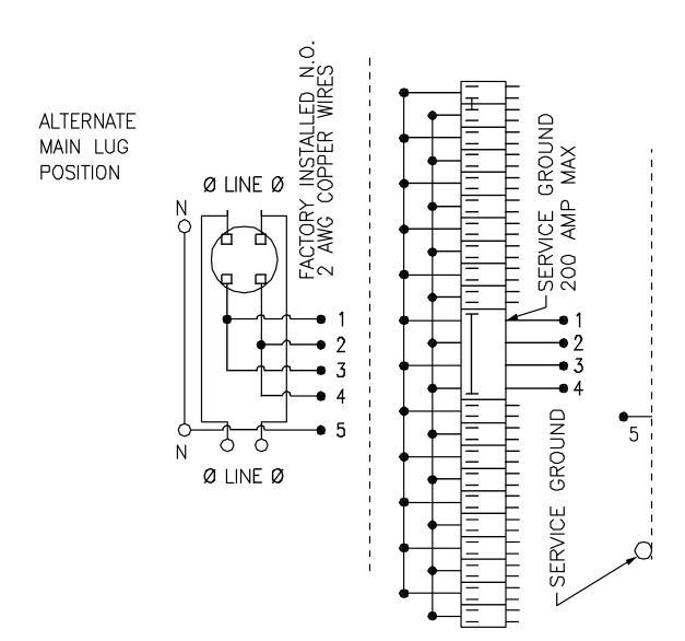
TWO SINGLE POLE, ONE PLUG-ON SPACE TYPE HOMT OR ONE SINGLE POLE, ONE PLUG-ON SPACE TYPE HOM. TWO POLE TYPE HOM, HOMA OR HOMT MAY PLUG-ON TWO ADJACENT SPACES. BRANCH BREAKER IS LIMITED TO 100A MAX.
