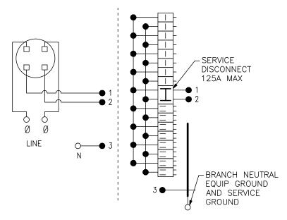
TWO SINGLE POLE, ONE PLUG-ON SPACE TYPE HOMT OR ONE SINGLE POLE, ONE PLUG-ON SPACE TYPE HOM. TWO POLE TYPE HOM, HOMA OR HOMT MAY PLUG-ON TWO ADJACENT SPACES. BRANCH BREAKER IS LIMITED TO 110A MAX.
