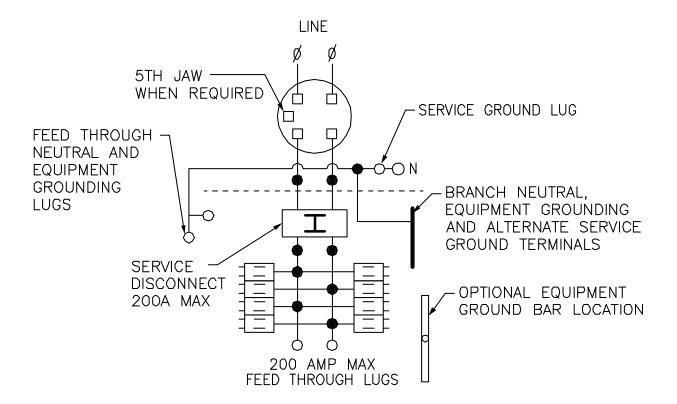
TWO SINGLE POLE, ONE PLUG-ON SPACE TYPE HOMT OR ONE SINGLE POLE TYPE HOM. TWO POLE TYPE HOM OR HOMT (15-100A) MAY PLUG ON TWO ADJACENT SPACES. TWO POLE HOMA (150-200A) MAY PLUG ON FOUR ADJACENT SPACES.
