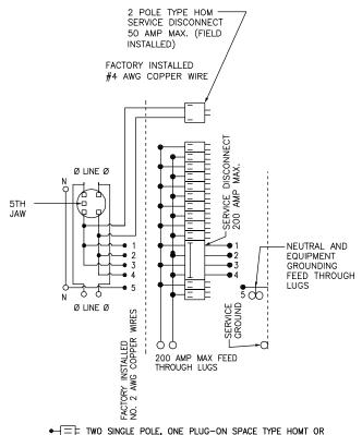
TWO SINGLE POLE, ONE PLUG-ON SPACE TYPE HOMT OR ONE SINGLE POLE, ONE PLUG-ON SPACE TYPE HOM. TWO POLE TYPE HOM, HOMA OR HOMT MAY PLUG-ON TWO ADJACENT SPACES. A 100 AMP MAX. CIRCUIT BREAKER MAY BE INSTALLED IN THE LOWEST POSITION IN THE BRANCH PANEL. ALL OTHER POSITIONS ARE LIMITED TO 70 AMP MAX. CIRCUIT BREAKERS.
