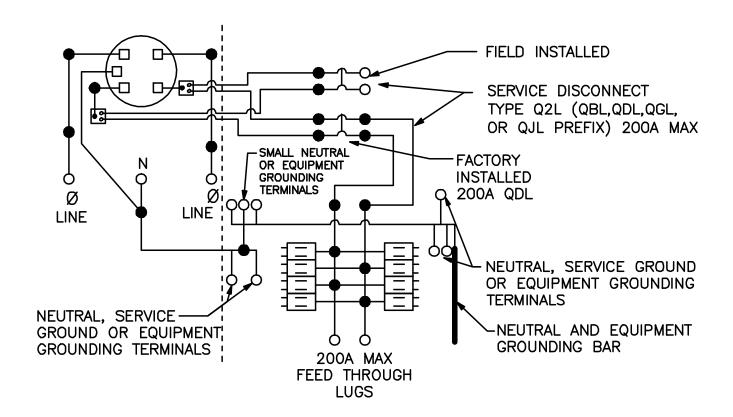
TWO SINGLE POLE, ONE PLUG-ON SPACE TYPE QOT OR ONE SINGLE POLE TYPE QO. TWO POLE TYPE QO, QOA OR QOC(125A MAX.) MAY PLUG-ON TWO ADJACENT SPACES. TWO POLE TYPE QOC (150-200A MAX.) MAY PLUG-ON FOUR ADJACENT SPACES (RIGHT SIDE ONLY).
