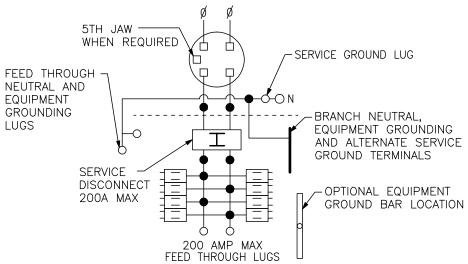
TWO SINGLE POLE, ONE PLUG-ON SPACE TYPE QOT OR ONE SINGLE POLE TYPE QO. TWO POLE TYPE QO OR QOA (15-100A) MAY PLUG ON TWO ADJACENT SPACES. TWO POLE TYPE QOC (150-200A) MAY PLUG ON FOUR ADJACENT SPACES. USE 10-100A AND 150-200A BRANCH BREAKERS ONLY.
