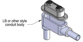
Remove existing Conduit Body cover and replace with Mencom Conduit Adapter.
