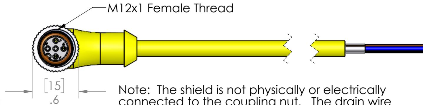
Note: The shield is not physically or electrically connected to the coupling nut. The drain wire is left long on the free end.
